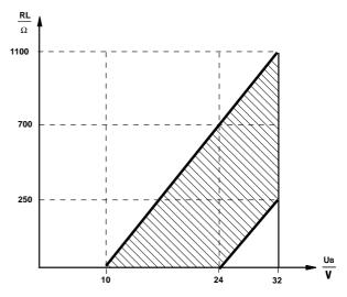
Max. Load: RL =  $\frac{\text{UB} - 10}{0.02 \text{ A}} \text{V}_{(\Omega)}$
