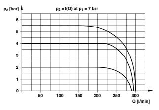
Flow characteristic with 7 bar operating pressure
