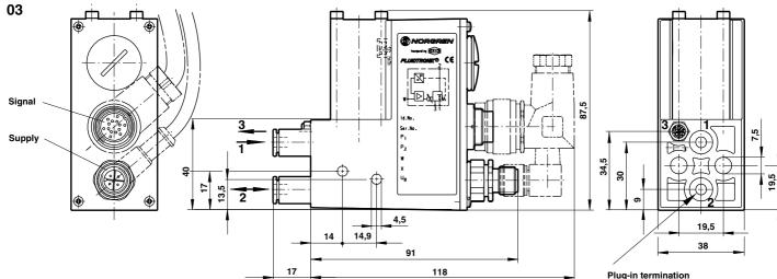
Plug-in termination for pipe OD = 6 mm
