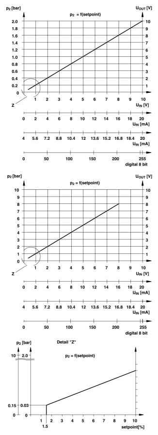
The valve function is activated as soon as the setpoint is  $\geq$ 1,5%
